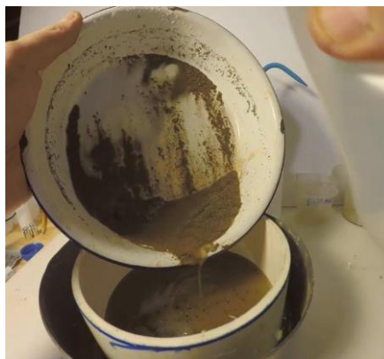
Figure 20. Transferring the material which passed the 2 mm sieve to the 250 micron sieve.
