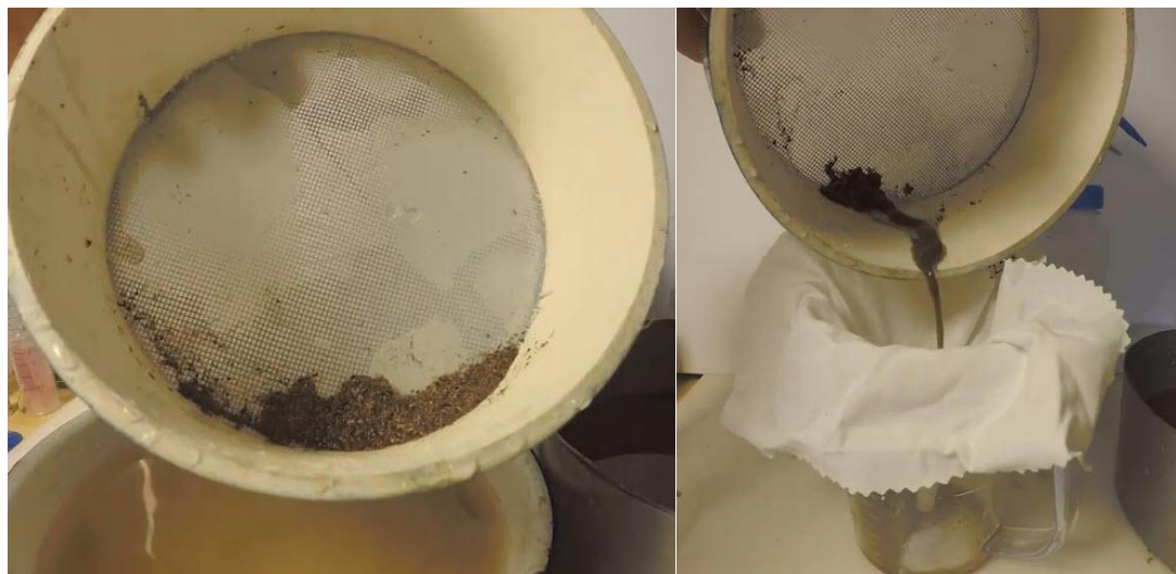
Figure 22. Left: POM that was decanted into the 250 micron sieve, at one side. Right: rinsing the POM onto a cloth or filter in a funnel, to later dry or score the amount captured.
