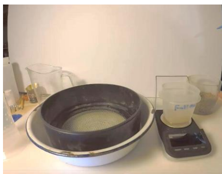
Figure 17. Preparing to wet-sieve the particulate organic matter (POM) out of soil, with the 2 mm sieve submerged in the pan of water.
