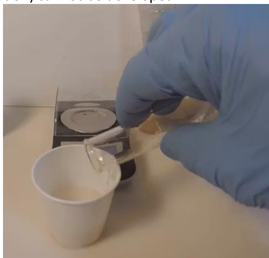
Figure 33. Mixing 3 mL solution of sodium bisulfate (15g \text{NaHSO}_4 per 100 mL) to acidify 7 mL of filtered extract. Note the bubbling of the soil extract as bicarbonate reacts with the acidic bisulfate.
