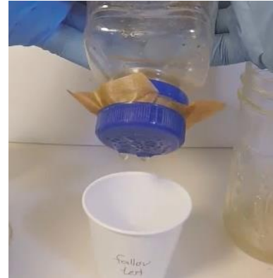
Figure 31. Pressing the bottle by hand to create a filtered soil extract.
