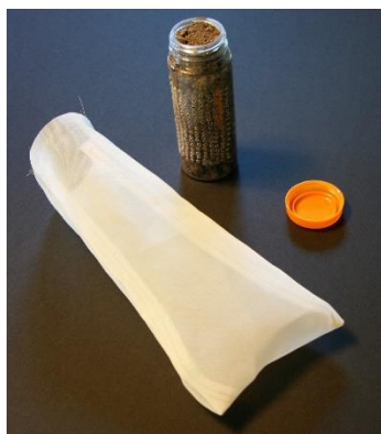
Figura R1. The mesh bag from 250 micron mesh and a bottle big enough for sieving 100g of soil, with 2mm holes drilled into the side of the bottle with a drill or hot nail.
