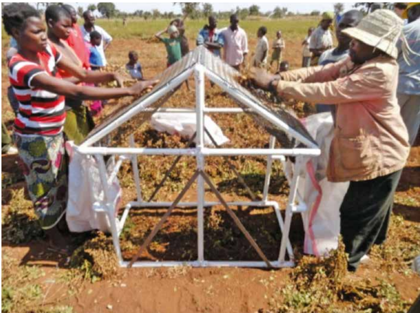
Stripping groundnuts with the A-frame fixed screen stripper
