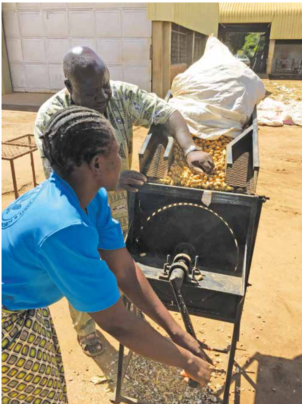
Shelling groundnuts with the mechanical sheller
