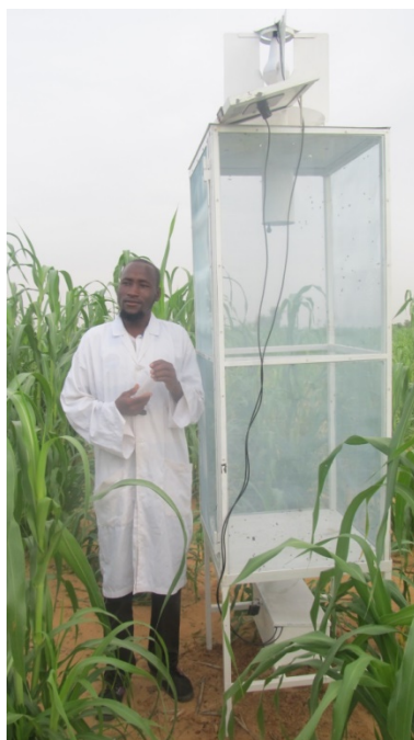
Solar light trap tested in Niger for MHW awareness system
