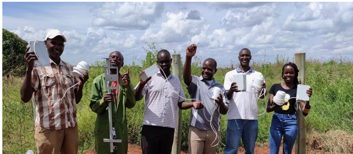
Installation of cheap, recyclable IoT rain gauges prototypes conceived by Manobi Africa and Viveris to reduce basis risk, insurance premiums and interest rates on smallholder credit. Photo: PCS Traore, ICRISAT Manobi Africa
