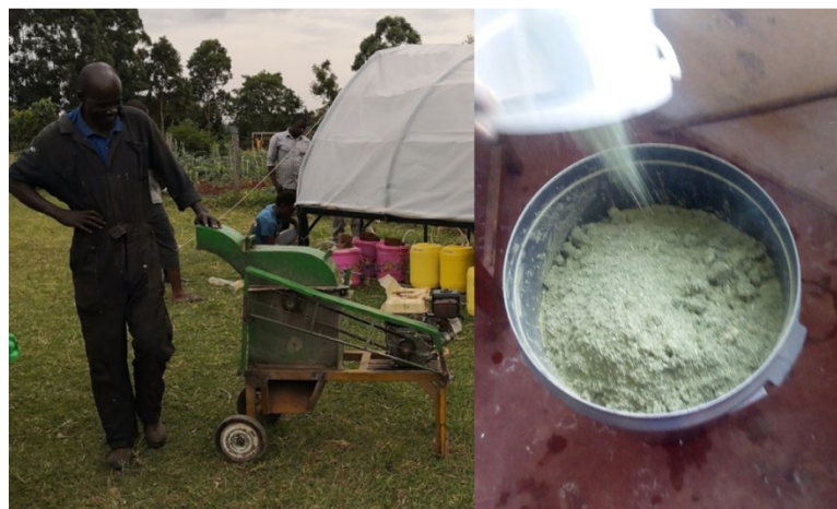
Figure 4: Left: Local residue-chopping machine that was able to grind the dried leaves to the desired consistency. Right: Resultant leaf powder being added to a container for making a pesticide solution.
